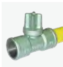
SERIES 451/73-001 Donkin Ball Valve Screwed to PE DN \frac{3}{4} "-2" / 25-63mm PN4 Ductile Iron Body Stainless Steel Ball GIS/V4 GIS/PL3
