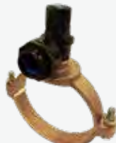
SERIES 1116/50-001 AC Self Tapping Saddle Saddle dia - 2"-12" Outlet - Pushfit d20-25mm WIS 4-22-02 Gunmetal saddle, stainless steel cutter, Acetal banjo and top cap
