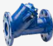
SERIES 53/35-003 AVK Flanged Ball Check Valve DN80-500 PN10/16 Ductile Iron EN 12050-4 BS EN 1092 (ISO 7005-2) DIN 3202-F6
