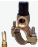
SERIES 1116/20-002 PVC Self Tapping Saddle BSP Saddle dia - d63-315mm Outlet - 1/2" - 1" BSP female WIS 4-22-02 Gunmetal saddle / banjo, DZR cutter and Acetal top cap
