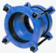
SERIES 602/1-001 AVK Universal Stepped Coupling DN63-400 PN16 Ductile Iron
