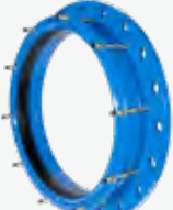
SERIES 260/30-001 AVK Fabricated Flange Adaptor DN300-1200 PN16 Mild Steel BS EN 1092 (ISO 7005-2)
