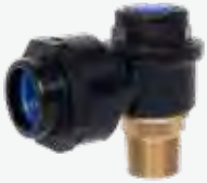
SERIES 1115/10-001 Swivel Ferrules Pushfit Inlet - 1/2"-3/4" Outlet - Push-fit d20-25 WIS 4-22-02 Gunmetal centre Acetal banjo and top cap
