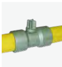
SERIES 451/70-001 Donkin Ball Valve with PE Tails DN25-63mm PN4 Ductile Iron Body Stainless Steel Ball GIS/V4 GIS/PL3
