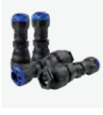
SERIES 1114/16-001 Universal Coupler Push-fit operation WIS 4-32-11 d20x15-22 to 50x49-63 PN16 Polycetal glass body Liner Series 1114/18
