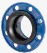
SERIES 05/26 AVK Combi-Flange DN50-300 PN10/16 Ductile Iron Tensile for Ductile Iron pipes BS EN 1092-2 (ISO 7005-2)
