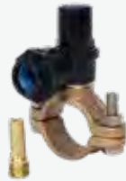
SERIES 1116/20-001 PE Self Tapping Saddle Saddle dia - d63-315mm Outlet - Pushfit d20 - 25mm WIS 4-22-02 Gunmetal saddle DZR cutter Acetal banjo and top cap
