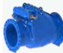
SERIES 41/39-001 AVK Free Shaft End Swing Check Valve, Metal seated DN50-300 PN16 Ductile Iron BS EN 1074-3 / EN 558 series 48 BS EN 1092-2 (ISO 7005-2)
