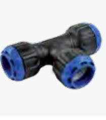
SERIES 1114/08-001 Equal Tee Push-fit operation WIS 4-32-11 d20x20x20-32x32x32 PN16 Polycetal glass body Liner Series 1114/18
