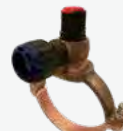
SERIES 1116/50-001 AC Self Tapping Saddle Saddle dia - 2"-12" Outlet - Pushfit d20-25mm WIS 4-22-02 Gunmetal saddle, stainless steel cutter, Acetal banjo and top cap
