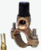
SERIES 1116/30-002 PVC Self Tapping Saddle BSP Saddle dia - 2"-12" Outlet - 1/2" - 1" BSP female WIS 4-22-02 Gunmetal saddle / banjo, DZR cutter and Acetal top cap 1/2" - 1" BSP
