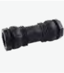
SERIES 1114/02-001 Repair Coupler Push-fit operation WIS 4-32-11 d20-50 PN16 Polycetal glass body Liner Series 1114/18 Threads female taper R
