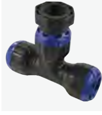
SERIES 1114/09-001 Tee Female Push-fit operation WIS 4-32-11 d25x3/4"-32x1" PN16 Polycetal glass body Threads female taper Rp Liner Series 1114/18
