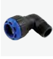
SERIES 1114/12-001 90° Male Elbow Push-fit operation WIS 4-32-11 d20x1/2"-32x1" PN16 Polycetal glass Threads male taper R Liner Series 1114/18
