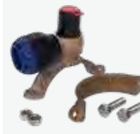
SERIES 1116/20-001 PE Self Tapping Saddle Saddle dia - d63-315mm Outlet - Pushfit d20 - 25mm WIS 4-22-02 Gunmetal saddle DZR cutter Acetal banjo and top cap
