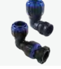
SERIES 1114/11-001 90° Female Elbow Push-fit operation WIS 4-32-11 d25x3/4"-32x1" PN16 Polycetal glass body Threads female taper Rp Liner Series 1114/18
