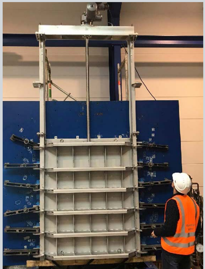
Penstock undergoing Factory Acceptance Testing
