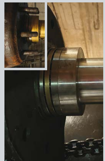
New Stainless Steel Spindle complete with thrust bearing assembly
