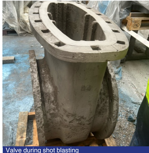
Valve during shot blasting
