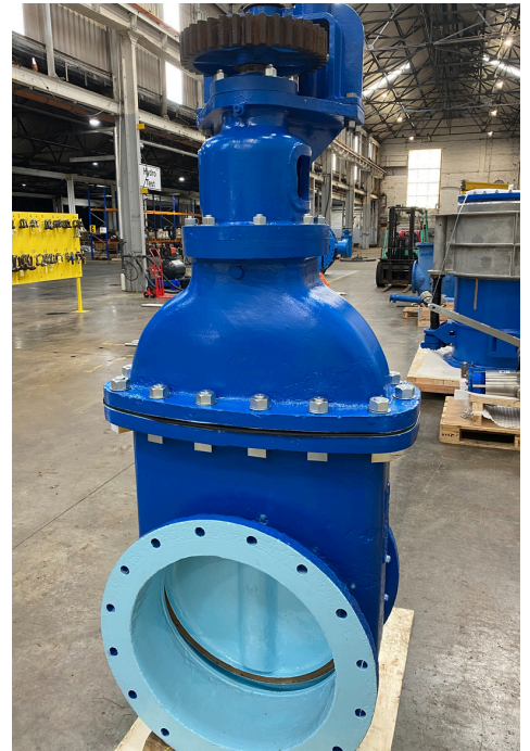
Final refurbished valve
