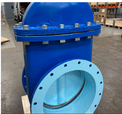
Final refurbished valve
