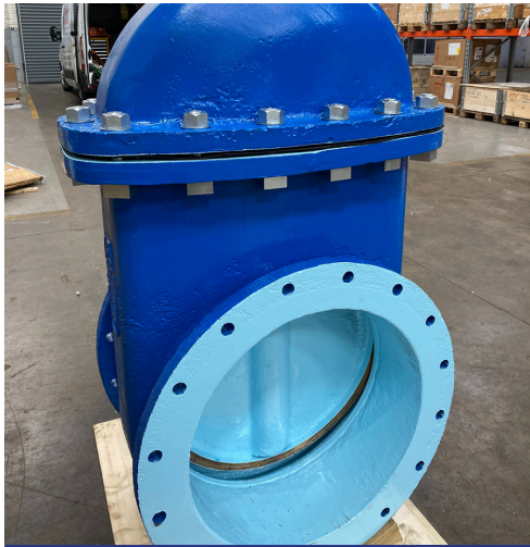
Final refurbished valve
