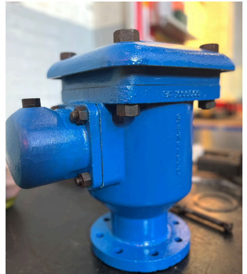
The refurbished air valve
