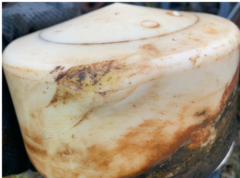
The original air valve
